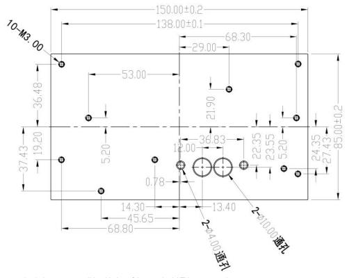
Note: Unit is mm. The mounting holes are compatible with that of the standard ATX power supply.
