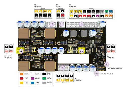
Note: J4 4-pin connector is for UART communication for power supply status monitoring. J5 4-pin connector is for synchronization between power supplies.
